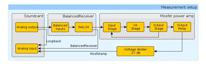
At three positions in the chain, the results are measured:
